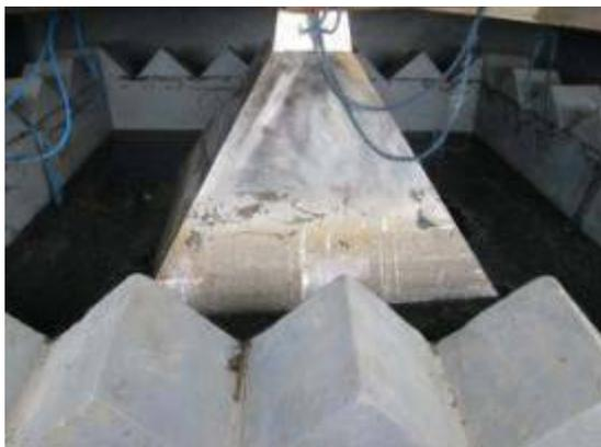
GLS (Gas Liquid Solid Separator)
