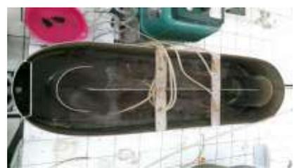
Reaktor Activated Sludge
